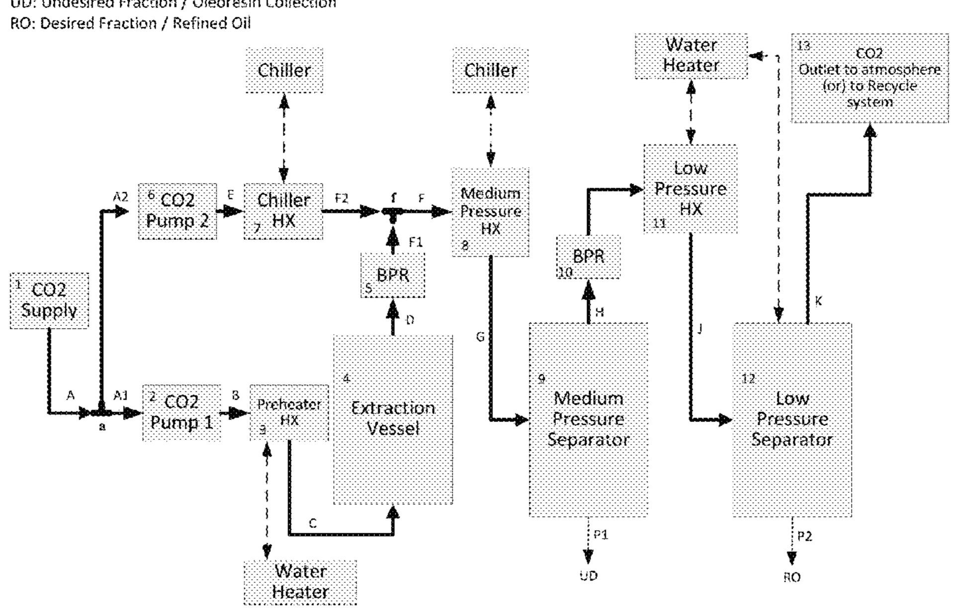
UD: Undesired Fraction / RO: Desired Fraction / Supply
