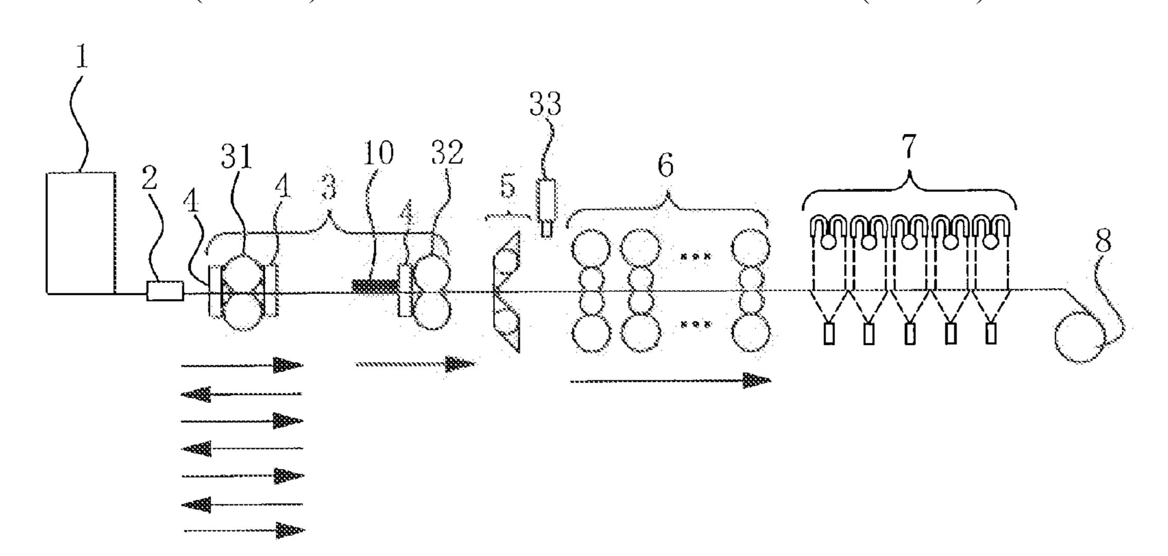
cooling at a water volume density of not less than 1000 L/min·m<sup>2</sup> and the other of the slow cooling apparatus and rapid cooling apparatus on a downstream side of the reversible rolling mill.
