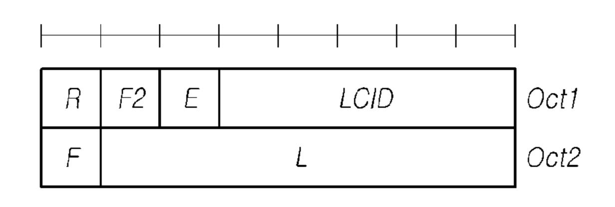
R/F2/E/LCID/F/L sub-header with 7-bits L field
