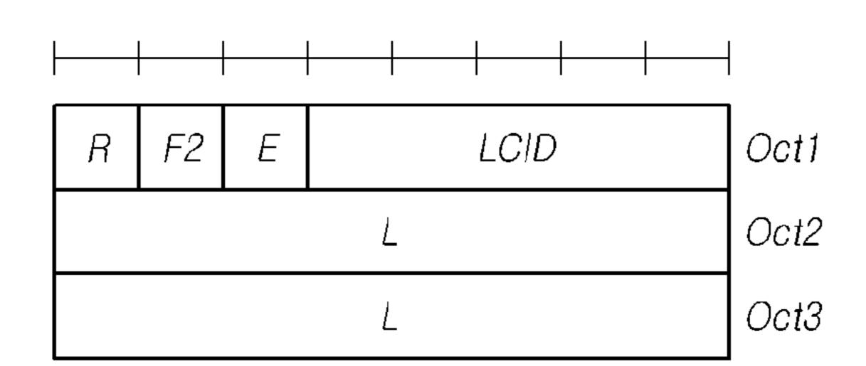
R/F2/E/LCID/F/L sub-header with 16-bits L field
