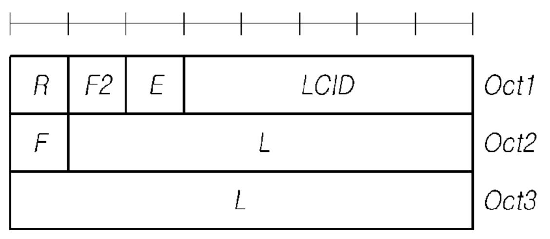
R/F2/E/LCID/F/L sub-header with 15-bits L field
