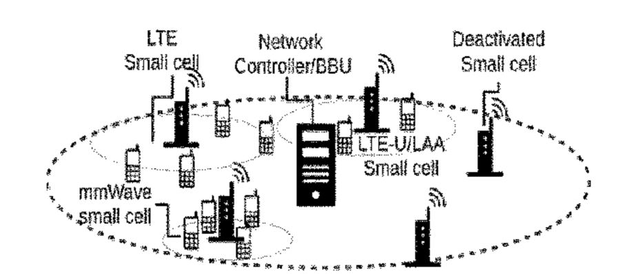
straints of the multi-RAT wireless communication network are defined and network constraint information is provided. Based on the queue information and the network constraint information, a resource scheduling algorithm is executed that jointly determines: an allocation of physical resource blocks (PRBs) to each link between a RAT and a mobile terminal, an assignment of modulation levels to each of the allocated PRBs, and an activation/deactivation of each of the RATs.
