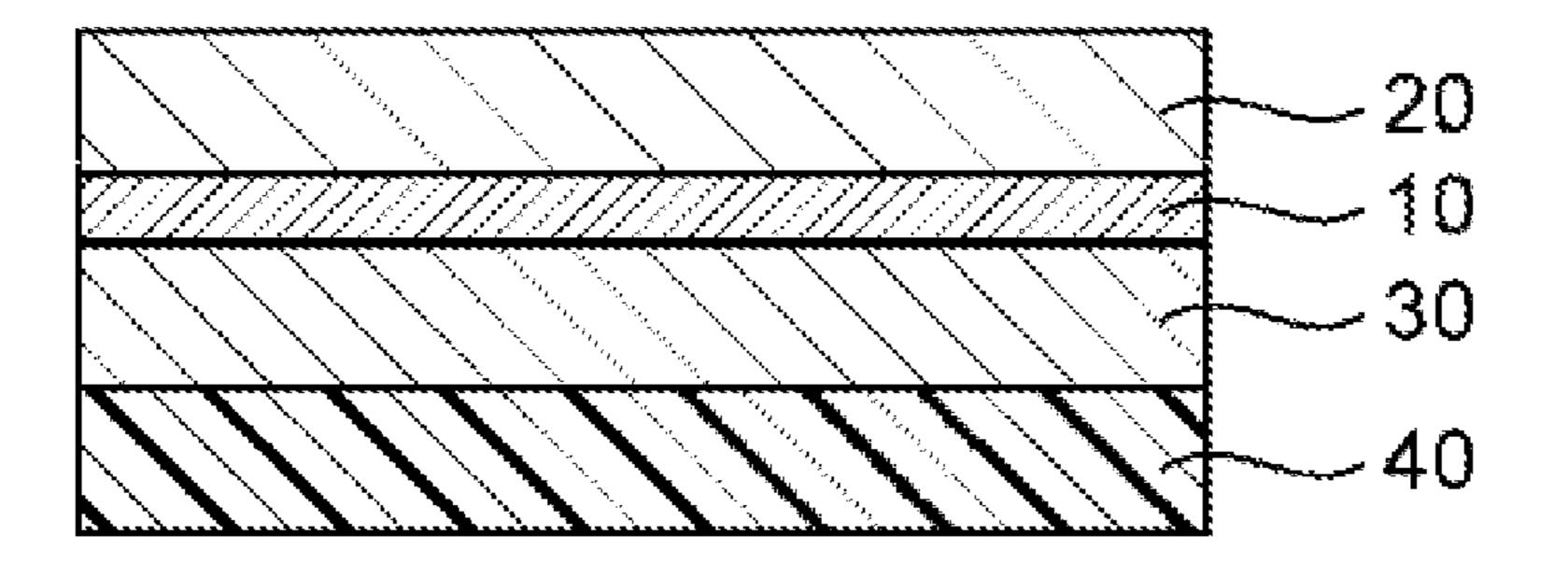
and has an Re (550) of from 230 nm to 310 nm. The second optical compensation layer shows a refractive index characteristic of nx>nz>ny and satisfies a relationship of Re (450)<Re (550).
