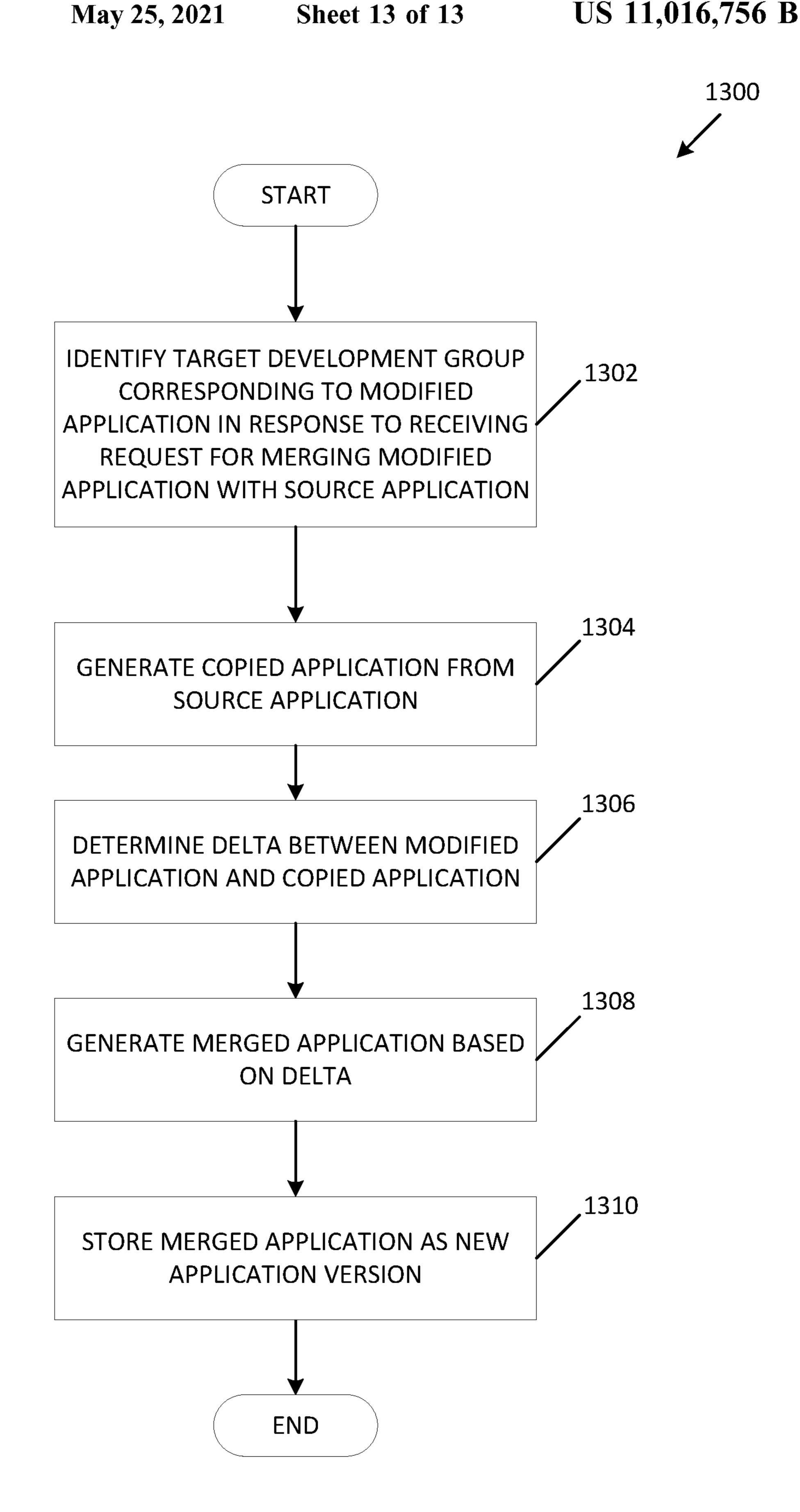
FIG. 13: EXEMPLARY APPLICATION MERGING PROCESS
