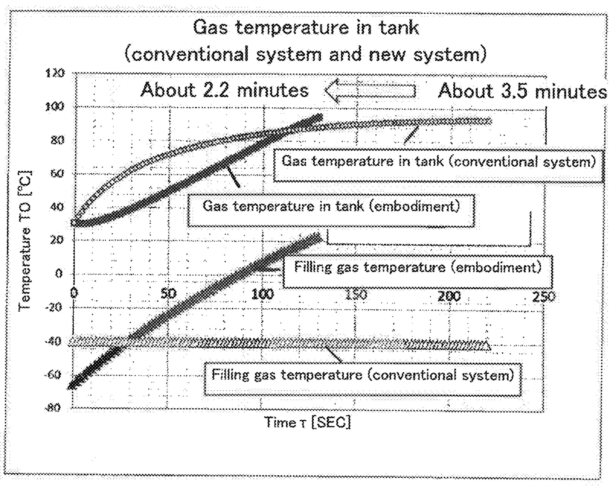
Tank capacity: 156L hydrogen gas main pressure: 82MPa(A), temperature: 30°C Initial tank pressure: 8MPa(A), initial tank temperature: 30°C
