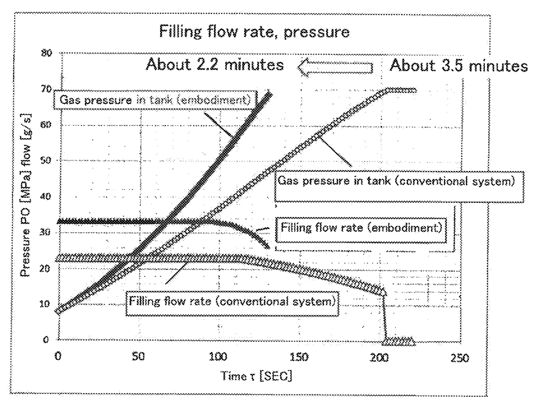
Tank capacity: 156L hydrogen gas main pressure: 82MPa(A), temperature: 30°C Initial tank pressure: 8MPa(A), initial tank temperature: 30°C
