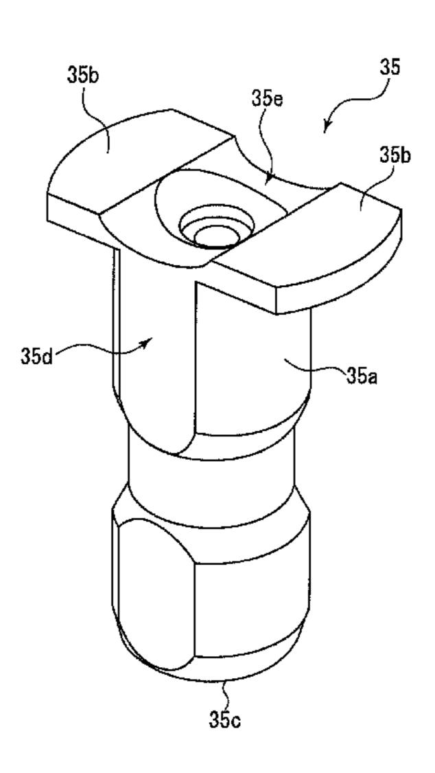
surface of the opposing groove portion formed in a symmetrical arc shape as viewed in the radial direction.
