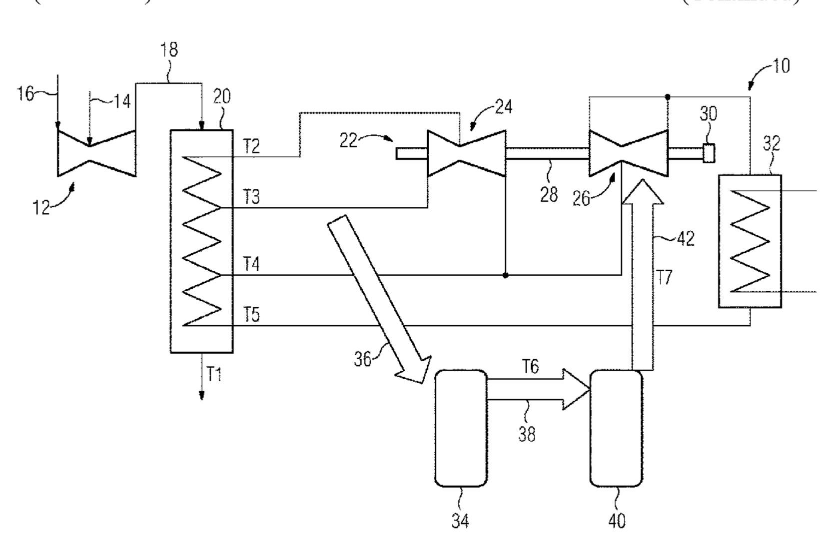
discharging at least a part of the steam stored in the steam accumulator from the steam accumulator; heating the steam discharged from the steam accumulator with heat released during an exothermic chemical reaction; and feeding the heated steam to drive the turbine device.
