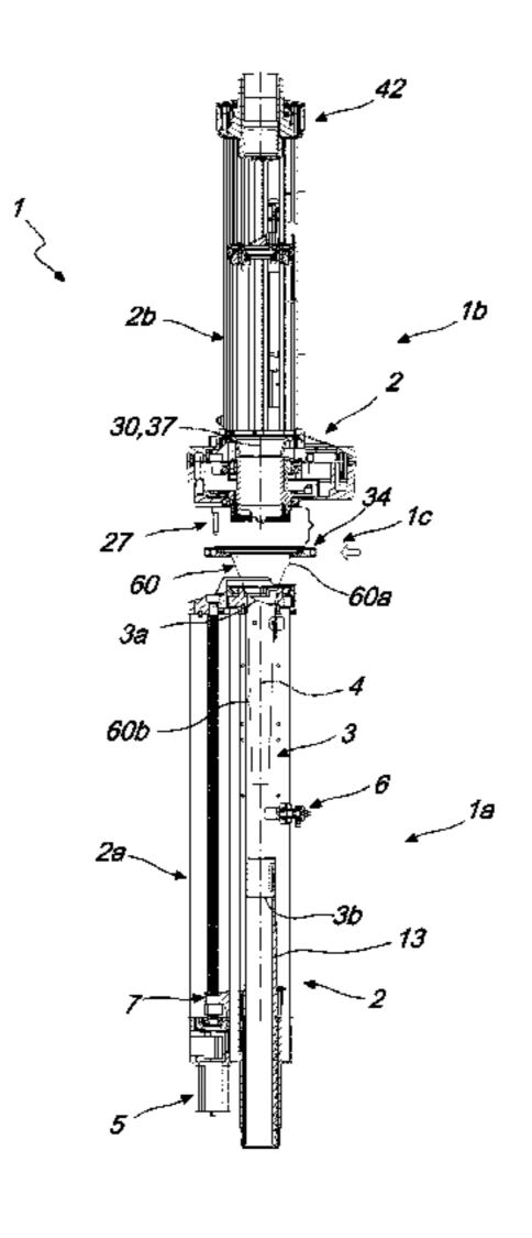
activated to perform a translation of the tubular body along its axis with respect to the main supporting structure. The tubular body is insertable, with its upper axial end, through an axial end of a tubular article in order to turn it inside out. The turning device comprises second actuation means which can be activated to rotate the tubular body about its own axis, through an angle of preset breadth, with respect to the main supporting structure.
