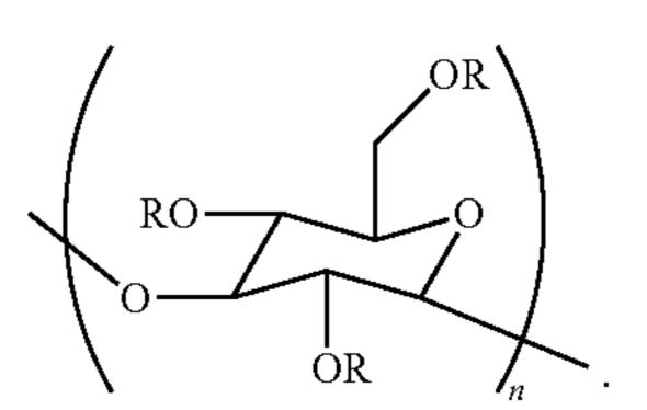
Regarding the formula of this structure, n can be at least 6, and each R can independently be an H or an organic group. Furthermore, the poly alpha-1,3-glucan ether compound has a degree of substitution with the organic group of about 0.05 to about 3.0.
