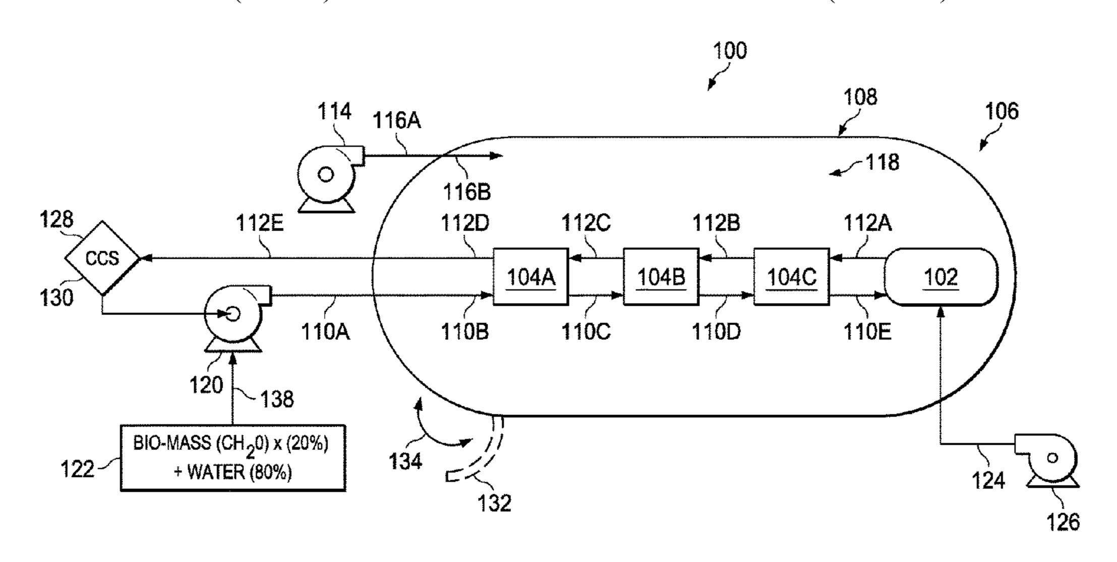
present invention allows the heat transfer function to be conducted independently from the pressure transfer function such that the system equipment can be designed and fabricated in manner that would support commercial scaled-up SCWG operations. By using heat exchangers coupled to the reactor in a series configuration, significant efficiencies are achieved by the present invention SCWG system over prior known SCWG systems.
