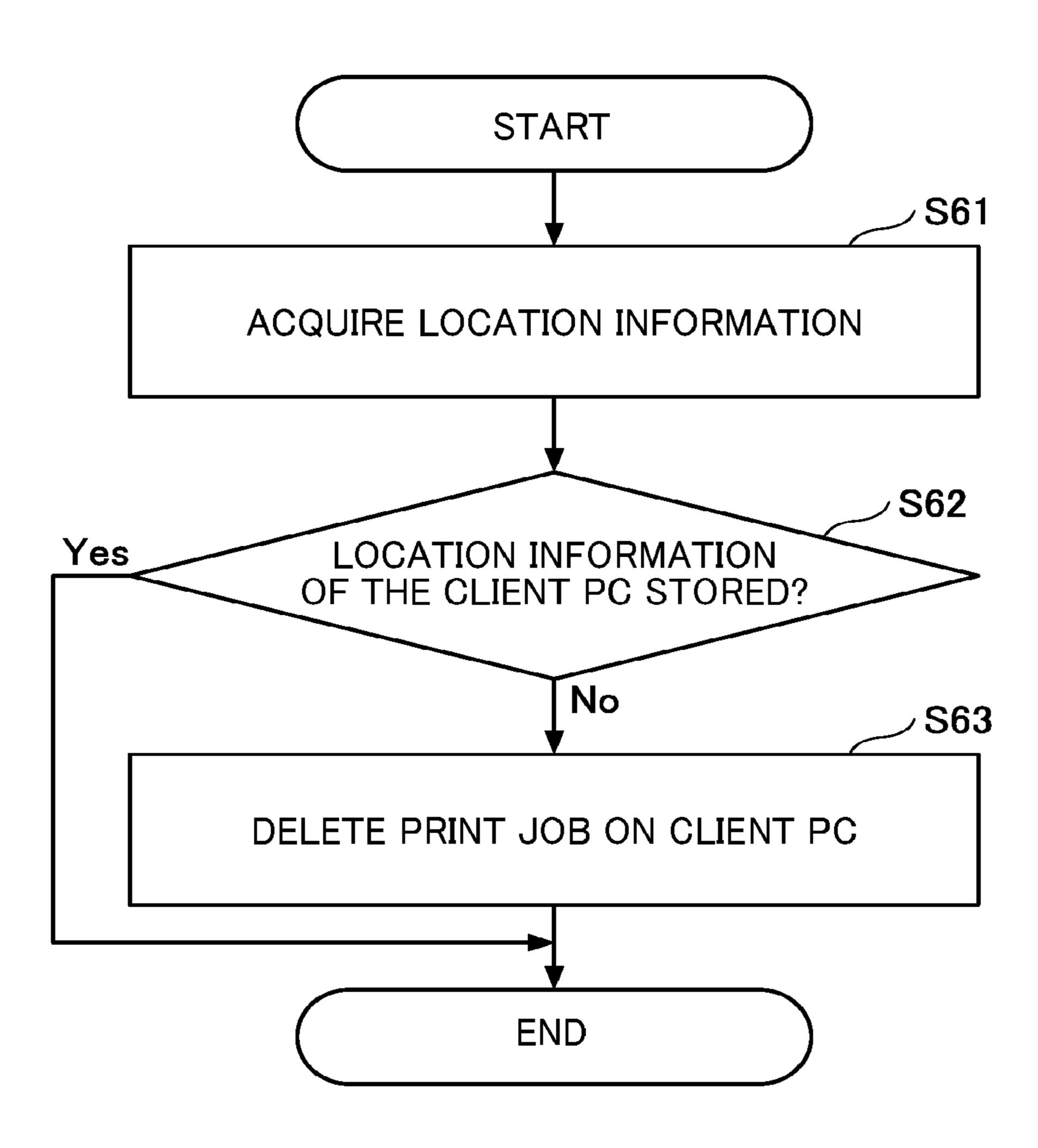
INFORMATION PROCESSING SYSTEM, INFORMATION PROCESSING APPARATUS, AND SERVER COMPRISING: PROCESSING CIRCUITRY CONFIGURED TO: STORE, IN A MEMORY OF THE SERVER, A PRINT JOB RECEIVED FROM AN INFORMATION PROCESSING APPARATUS THAT CREATES AND STORES THE PRINT JOB LOCALLY SO THAT THE PRINT JOB IS STORED BOTH IN THE MEMORY OF THE SERVER AND IN THE INFORMATION PROCESSING APPARATUS AT A SAME TIME
