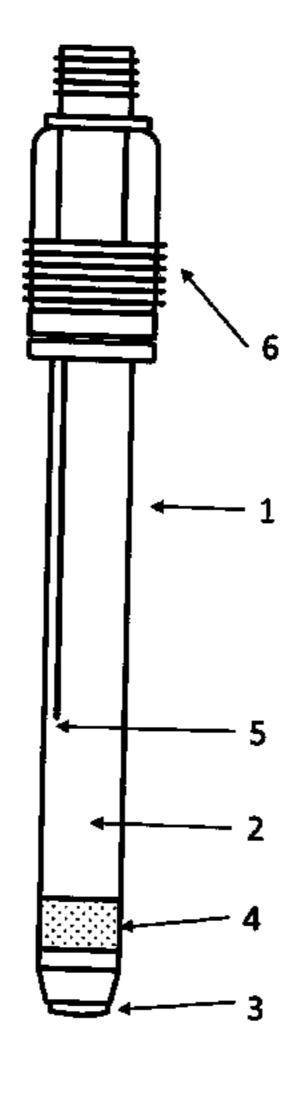
porous platinum membrane having a pore size of  $0.15~\mu m$  to  $0.25~\mu m$ , which produces the contact with the electrolyte and the water.
