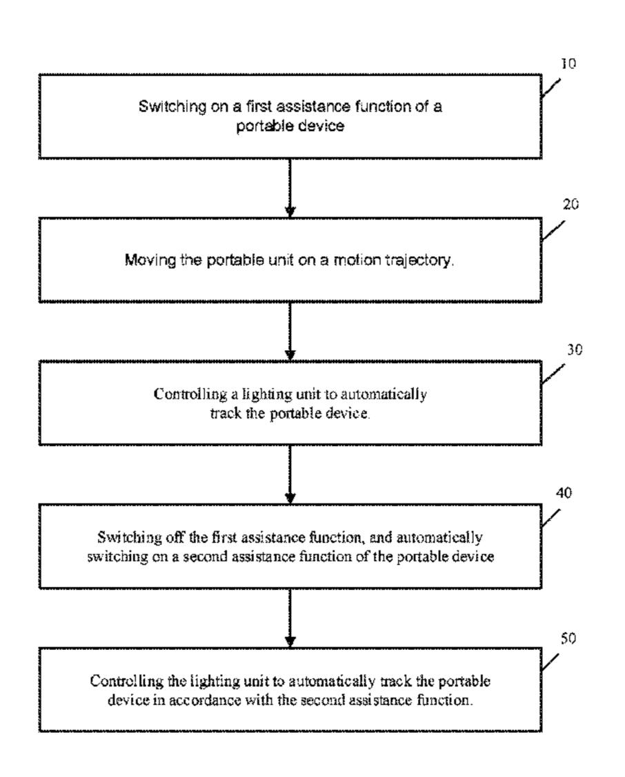
light beam emitted by the lighting unit automatically tracks the portable unit in accordance with the motion trajectory of the portable unit.
