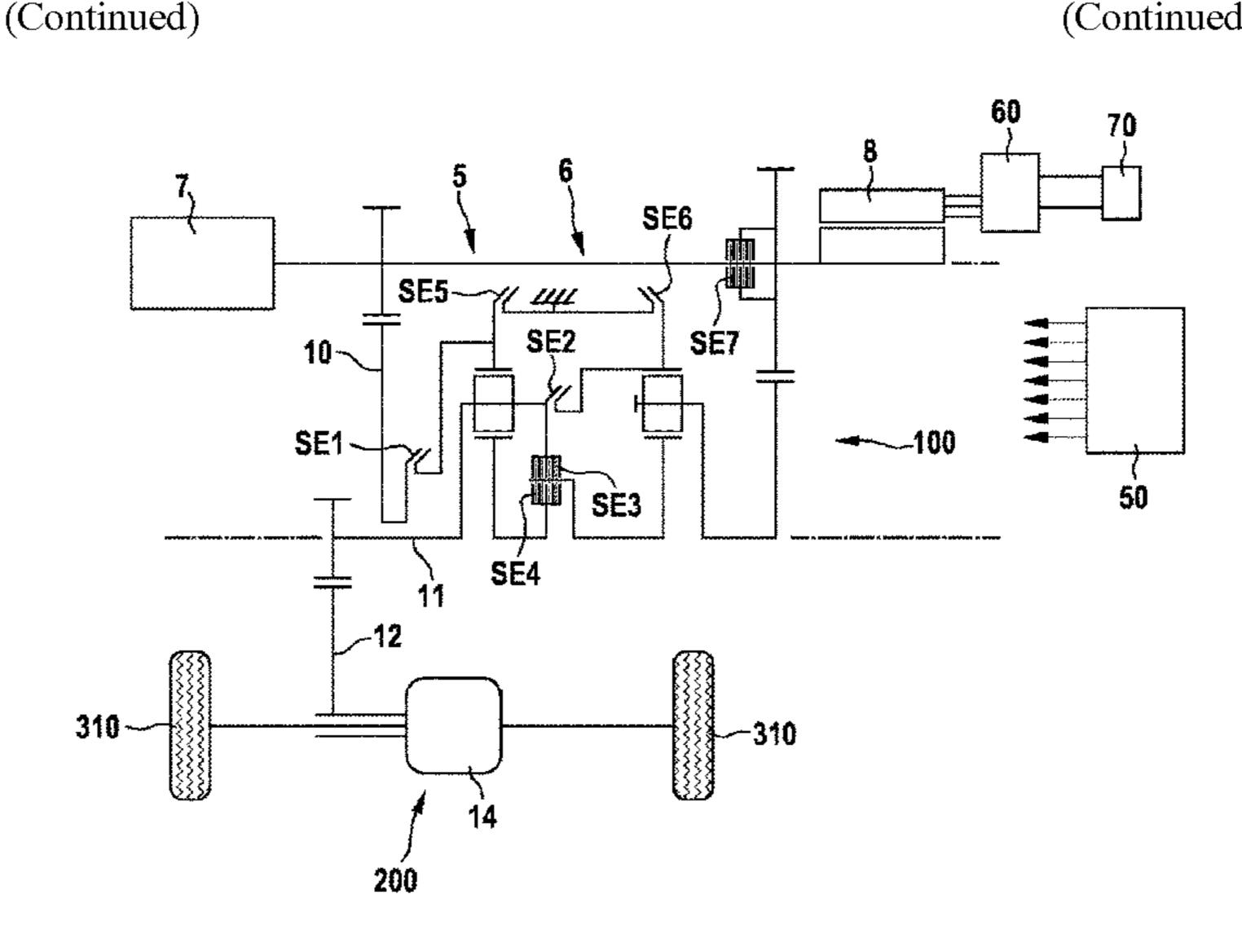
carrier of the first planetary gear (5) can be coupled to the ring gear of the second planetary gear (6) by means of the second shifting element (SE2) and the planet carrier of the first planetary gear (5) can be coupled to the sun gear of the second planetary gear (6) by means of the third shifting element (SE3). The sun gear of the first planetary gear (5) can be coupled to the sun gear of the second planetary gear (6) by means of the fourth shifting element (SE4).
