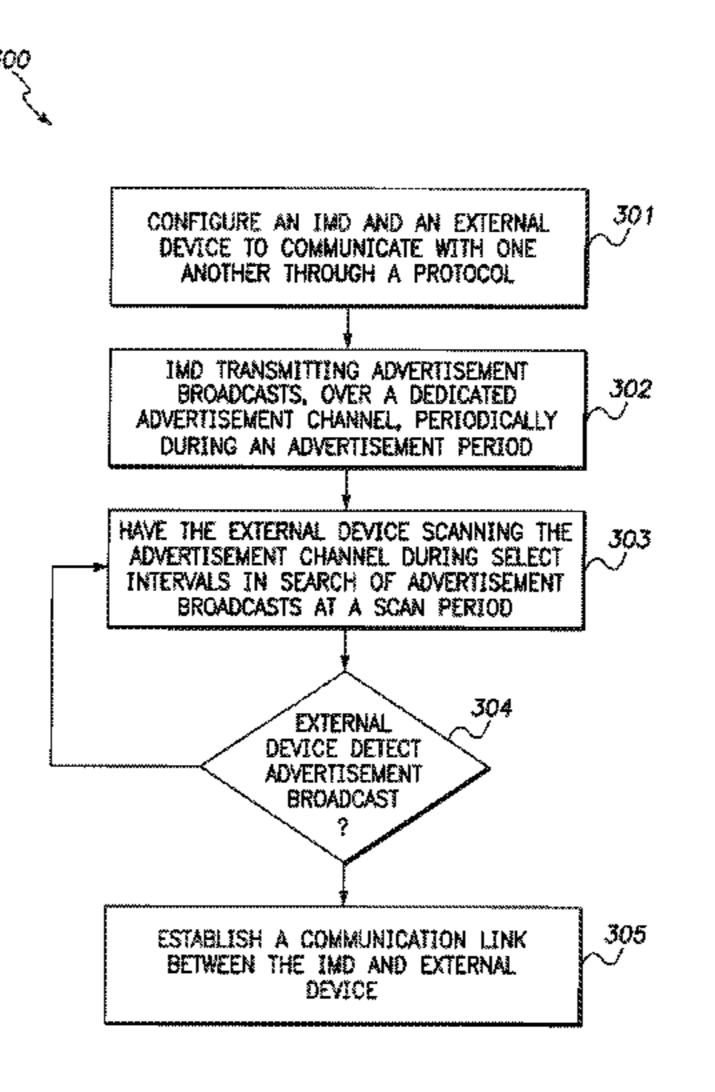
pendent of one another such that the advertisement and scan periods at least partially overlap intermittently after a number of cycles. When the external device detects one of the advertisement notices, the method includes establishing a communications link between the external device and the IMD.
