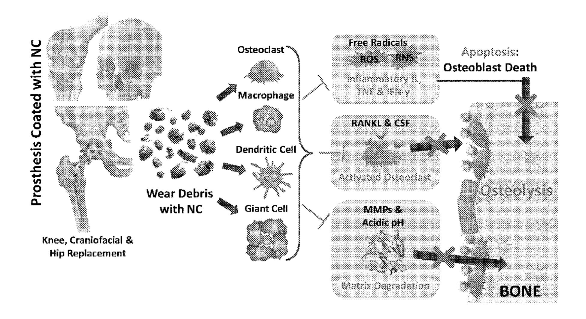
one or more nanoceria coatings exhibit catalase mimetic activity, superoxide dismutase mimetic activity, or both. Methods are provided for forming a nanoceria coaling. The coating has nanoceria having a surface cerium 3+/4+ oxidation state ratio such that such that the coating exhibits catalase mimetic activity, superoxide dismutase mimetic activity, or both. Also disclosed is a method of reducing degradation of an implant by placing nanoceria in proximity to a bone-implant interface.
