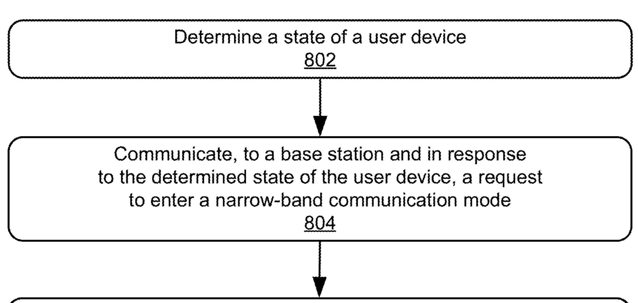
Receive, from the base station, an identification of selected resource elements for communication in the narrow-band communication mode that includes respective frequencies and time locations of the selected resource elements 806
