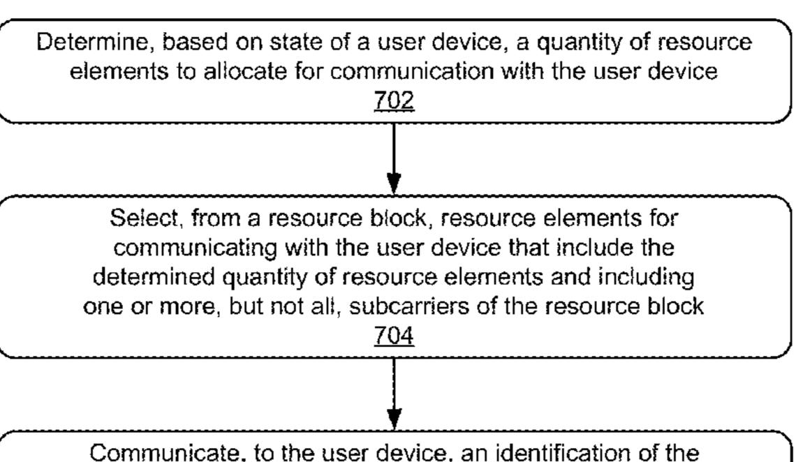
Communicate, to the user device, an identification of the selected resource elements including respective frequencies and time locations of the selected resource elements
