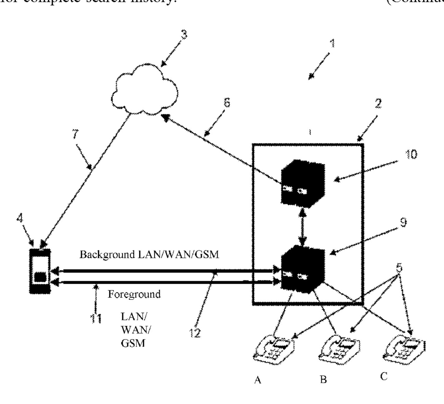
device is running in a background mode or in a foreground mode. When the PBX system determines that the application is running in the foreground mode, the PBX system uses the first connection for forwarding the call. When the PBX system determines that the application is running in the background mode the PBX system uses the second connection to receive information about the communication connection being used.
