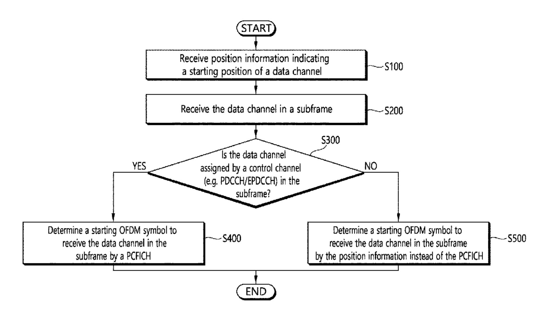
starts in the plurality of the downlink subframes is determined on the basis of the position information.
