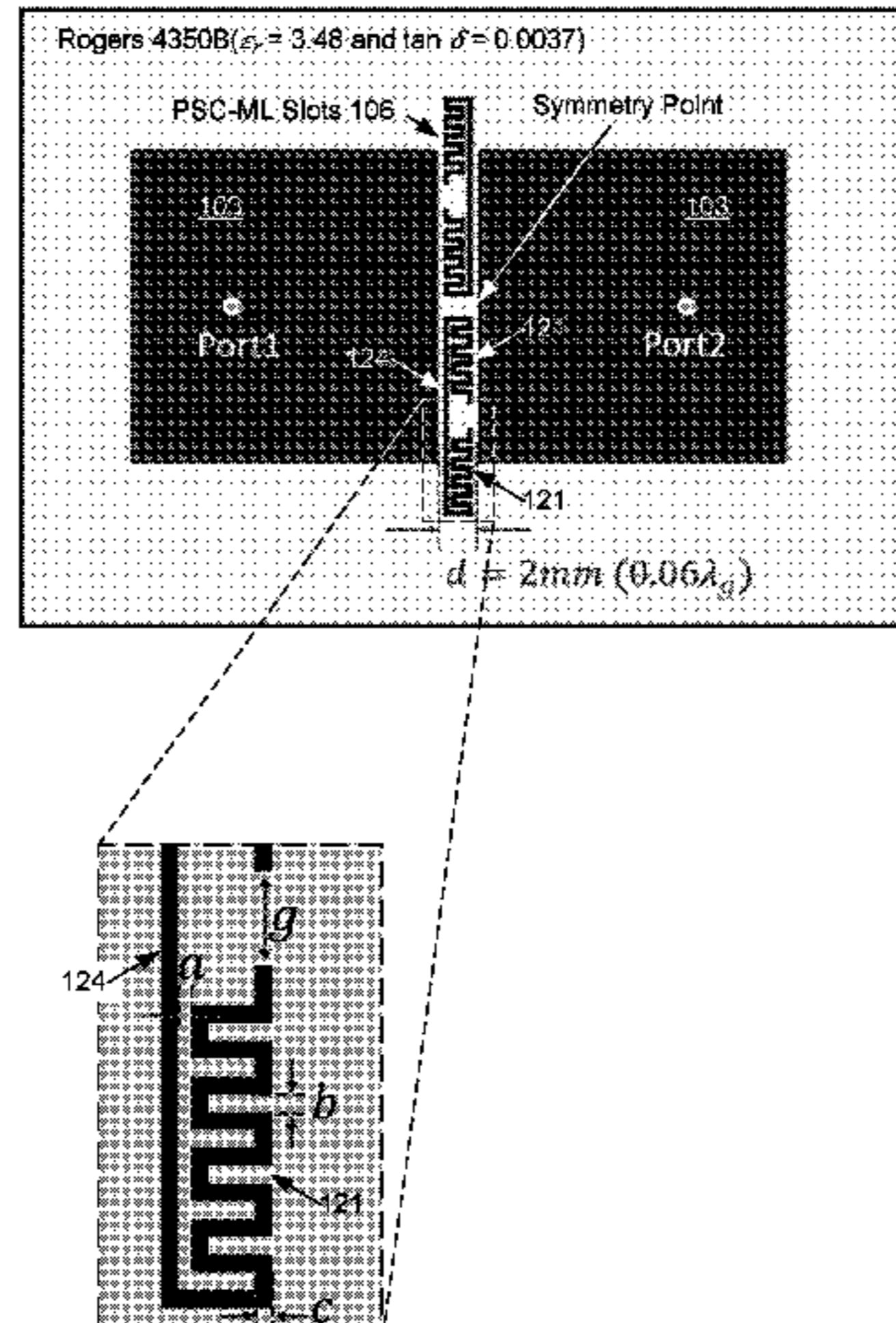
method includes forming first and second antenna elements on a first side of a substrate and forming PSC-ML slots in a ground plane disposed on a second side of the substrate that are aligned with a gap between the first and second antenna elements.
