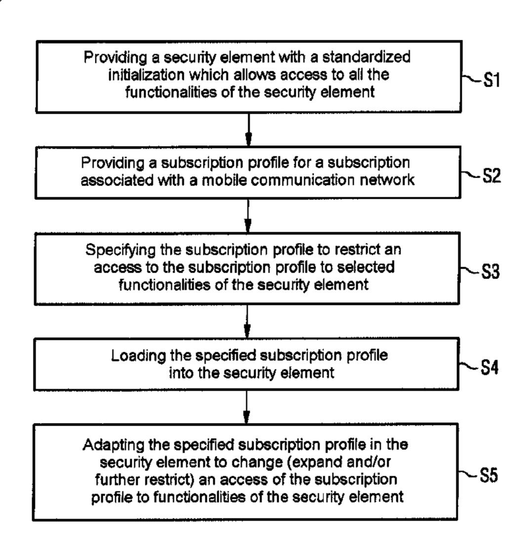
a subscription profile, an access to functionalities of the security element is subscription-profile-specifically restricted.
