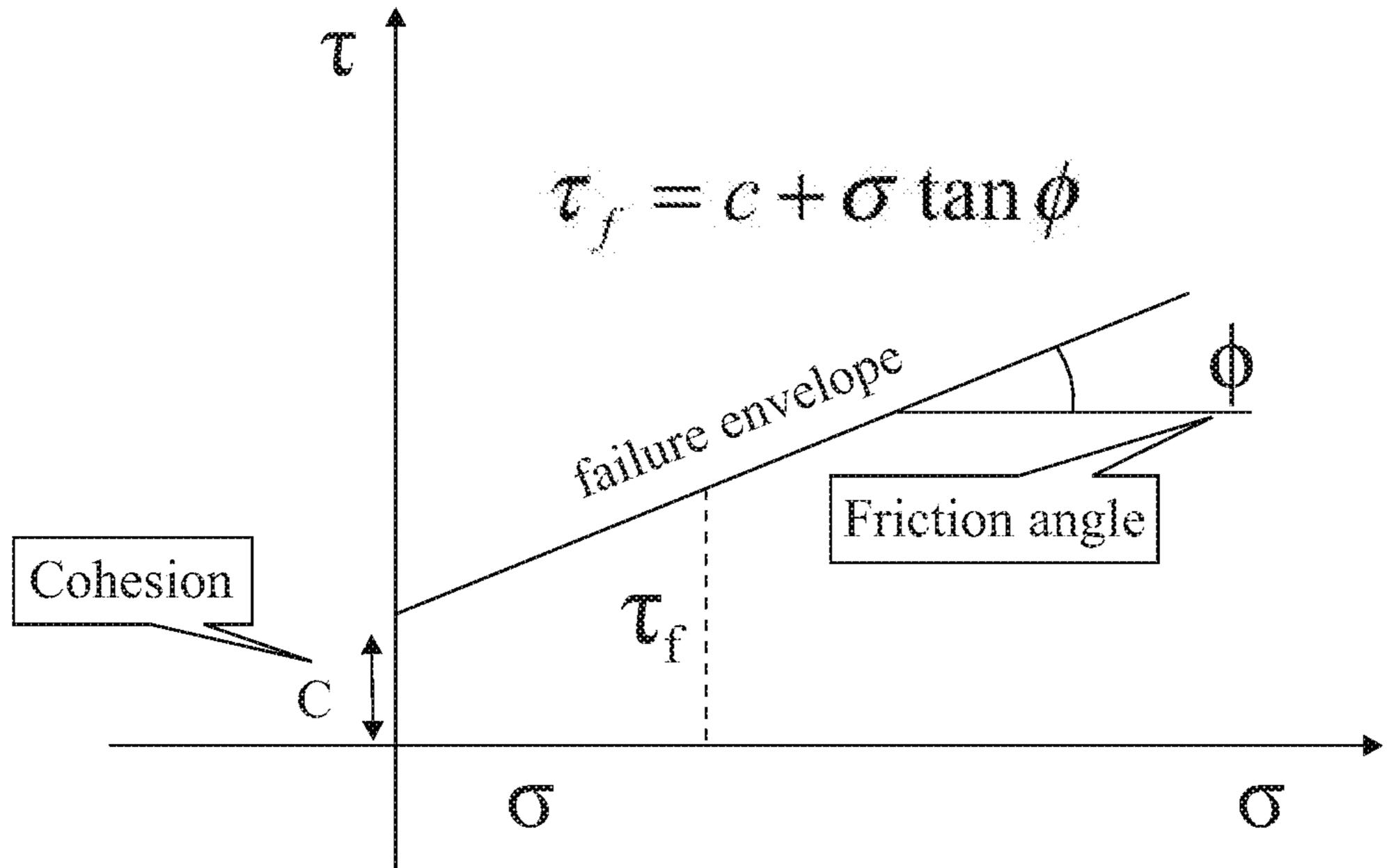
Tf is the maximum shear stress the soil can take without failure, under normal stress of **O**.
