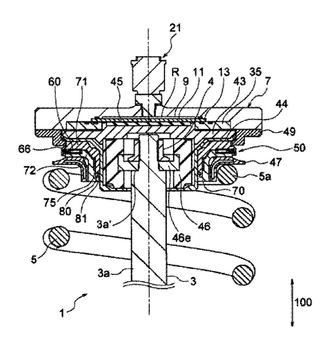
and receives a load in a radial direction while causing constant damping to swinging.
