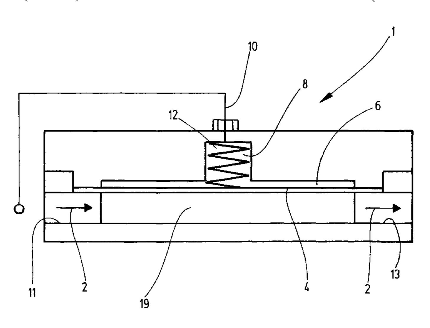
adjoins the fluid inlet (11) and the fluid outlet (13) and is delimited by at least one yielding wall part (4).
