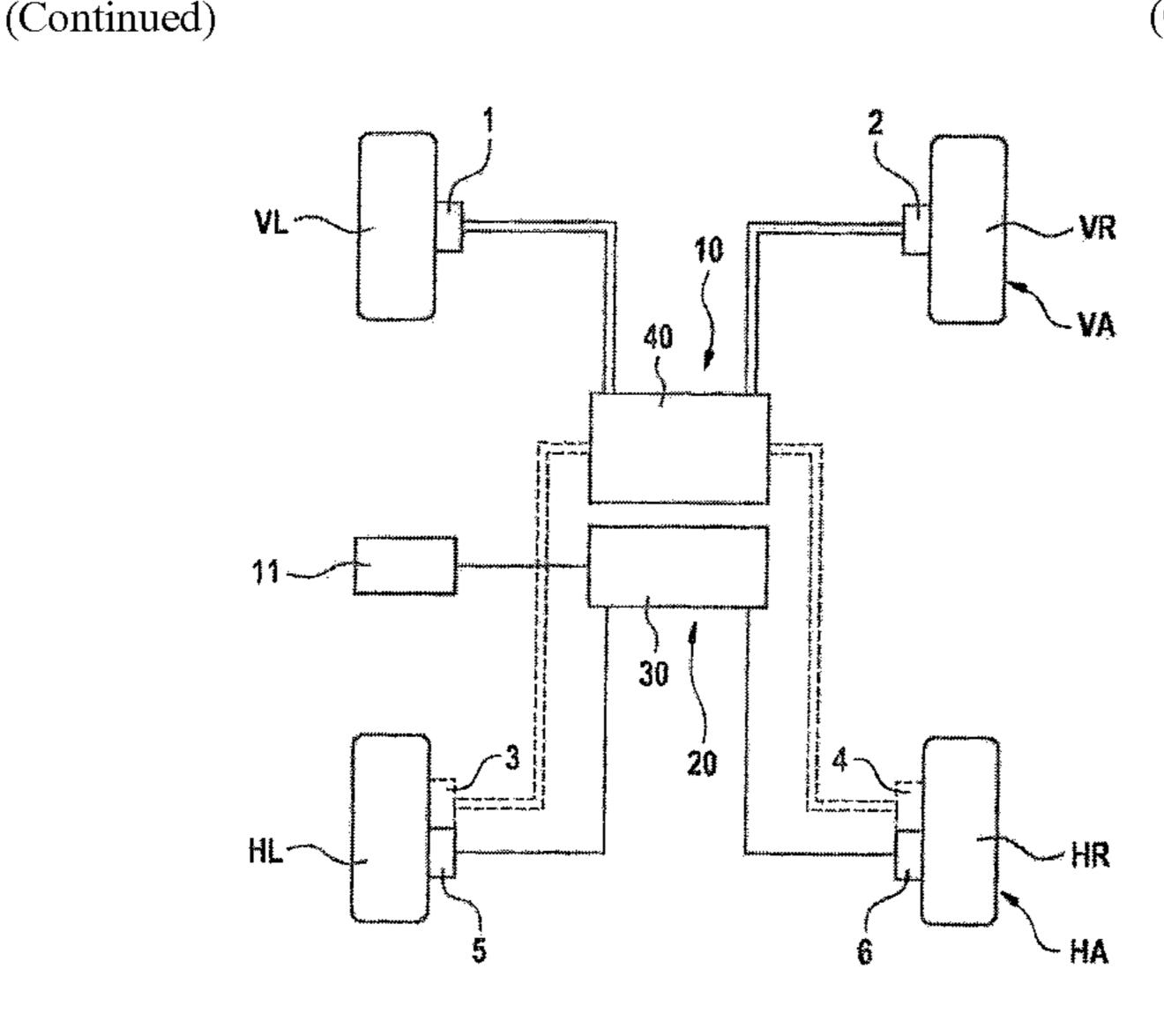
wherein a motor vehicle setpoint longitudinal deceleration which is to be achieved is determined, and the electromechanical actuators of the parking brake device are actuated in such a way that the motor vehicle actual longitudinal deceleration is adjusted to the motor vehicle setpoint longitudinal deceleration.
