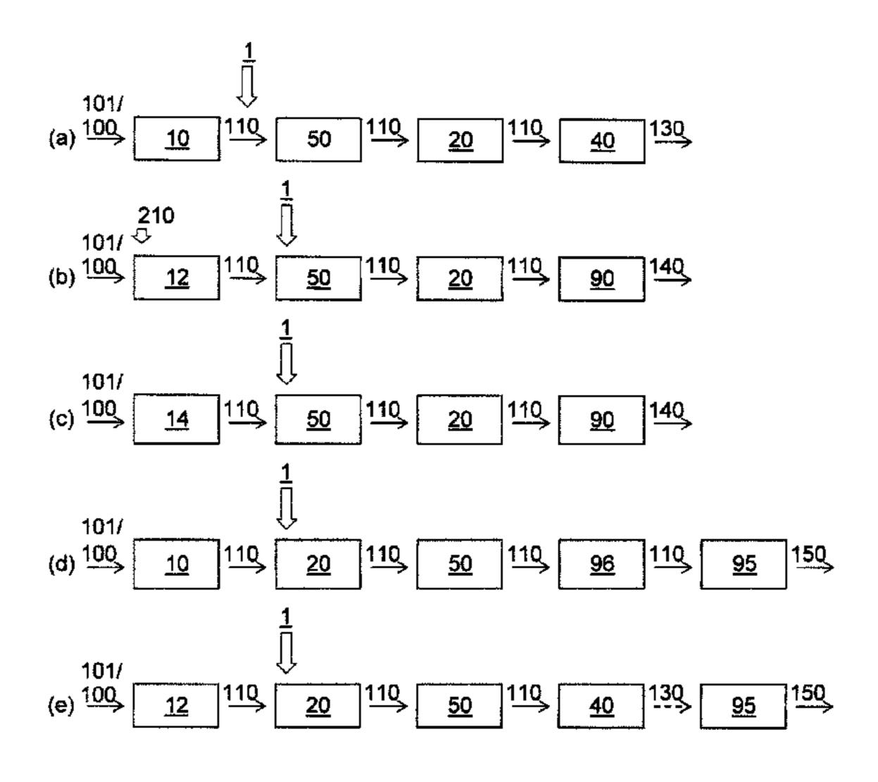
formed and expanded plastic material (140), and a molded expanded plastic article (150) obtainable by said process.
