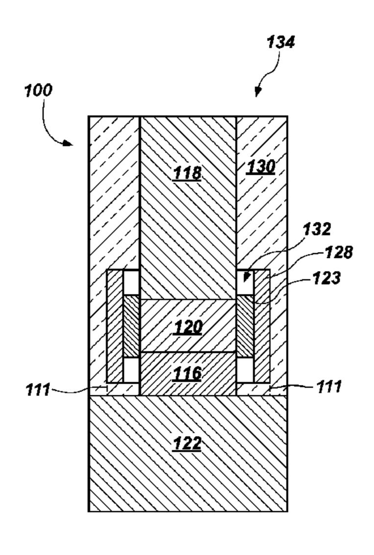
of the source region and the drain region of the semiconductive pillar. Related electronic systems and methods are also disclosed.
