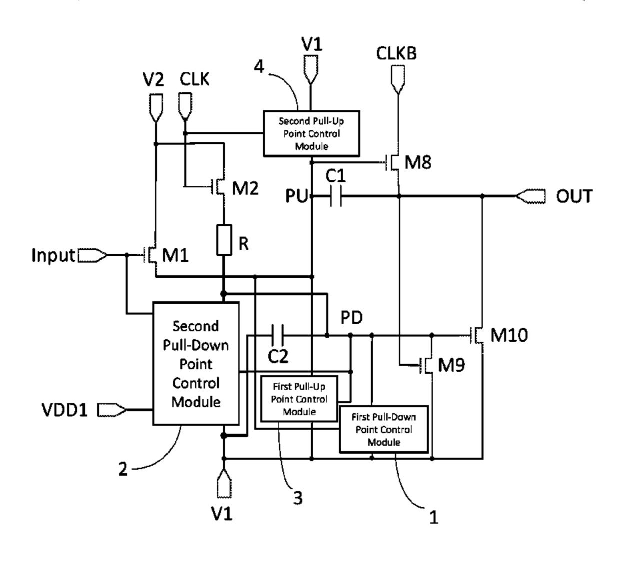
having a control end coupled to a first clock signal and two ends coupled to the pull-up point and the first voltage input respectively.
