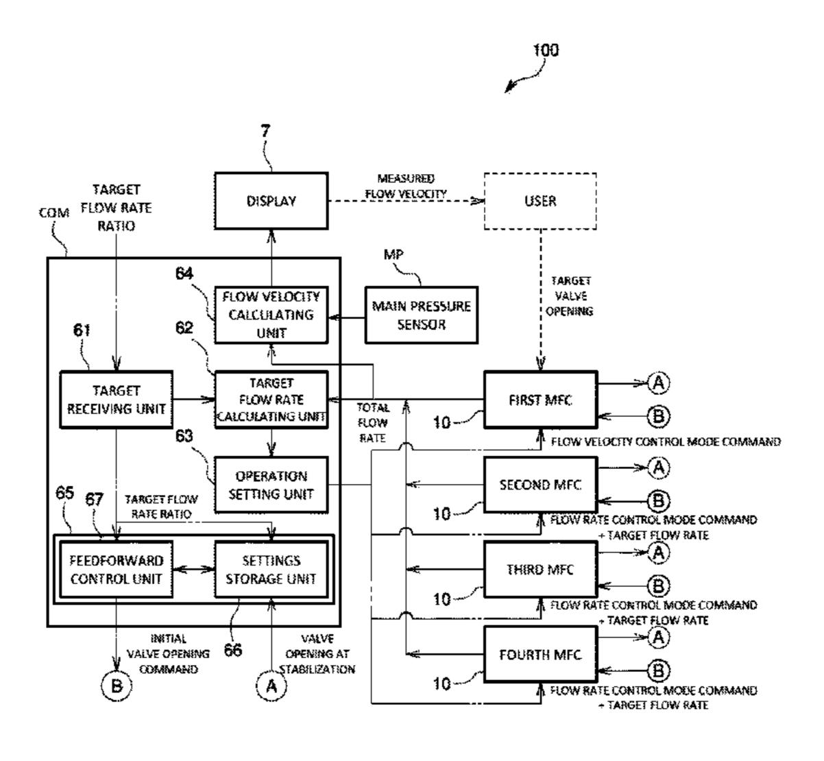
in which the flow velocity of a fluid is controlled upstream of each valve, and the remaining fluid control devices are made to operate in a flow rate control mode in which the flow rate is controlled based on the target flow rates.
