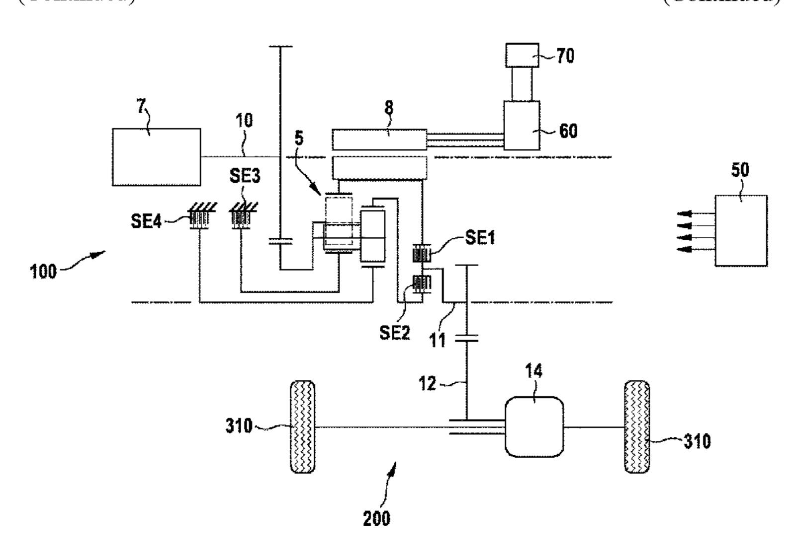
be coupled to the first ring gear of the double planetary gear (5) by means of the first shifting element (SE1) and can be coupled to the second ring gear of the double planetary gear (5) and by means of the second shifting element (SE2).
