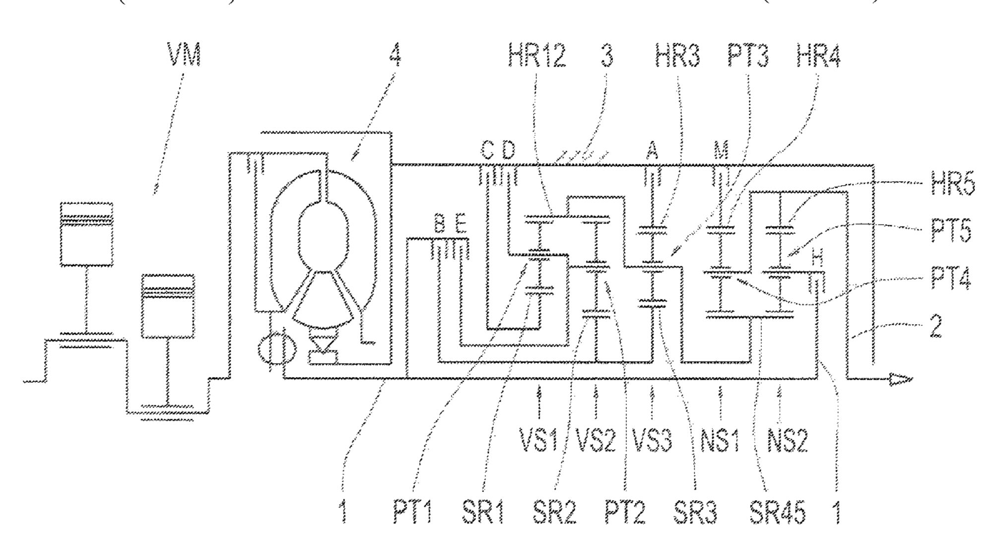
one output speed is greater than 1, one output speed is equal to 0, one output speed is equal to 1 and two output speeds are between 0 and 1.
