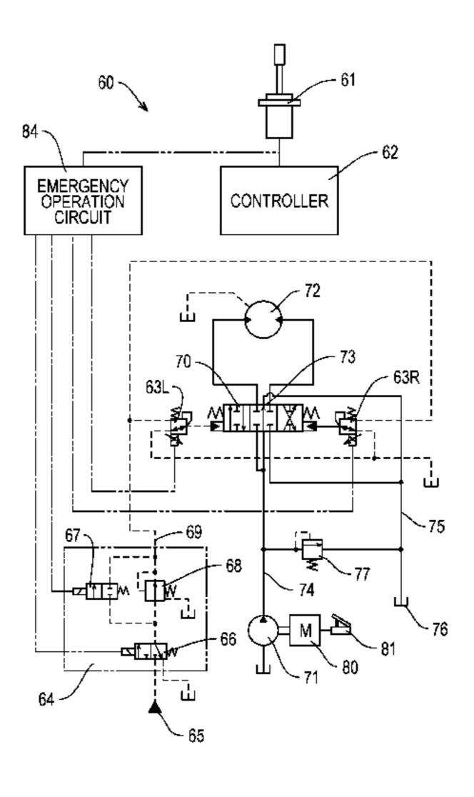
state, and the operating oil discharge amount from the hydraulic pump increases and decreases, and the operating oil pressure increases and decreases, and thus the operating speed of the actuator is controlled.
