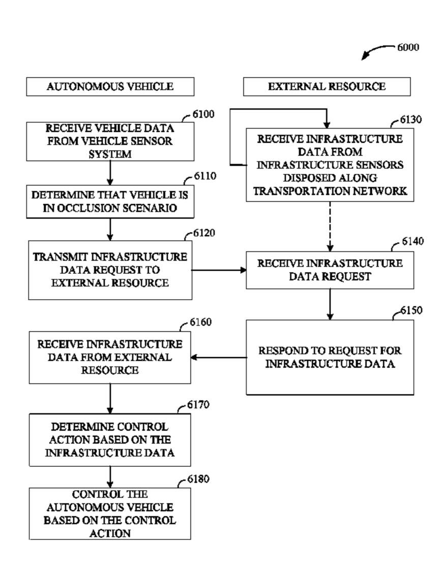
the vehicle sensor data, and controlling the autonomous vehicle based on the control action.
