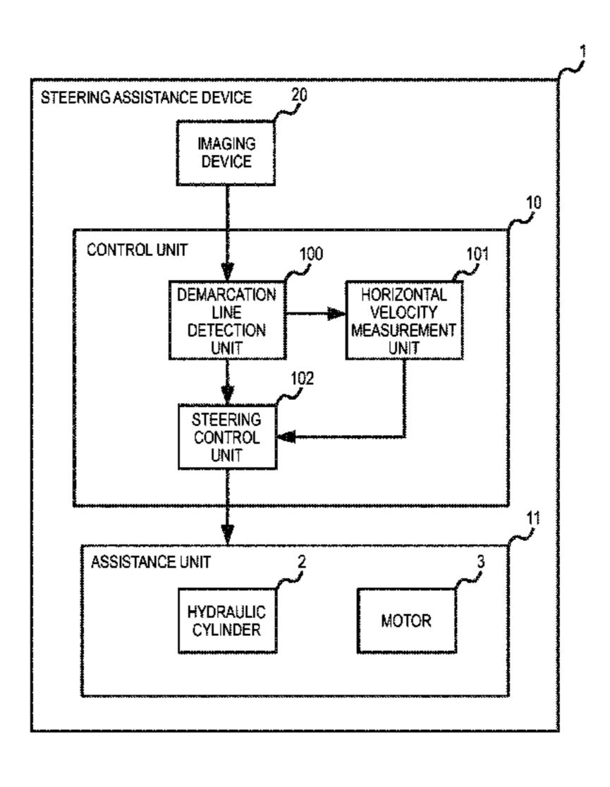
greater than a prescribed velocity and the center of the vehicle is separated from the center between the left and right lane demarcation lines by equal to or greater than a prescribed distance, a steering control unit 102 starts the steering assistance of the vehicle by the assistance unit 11.
