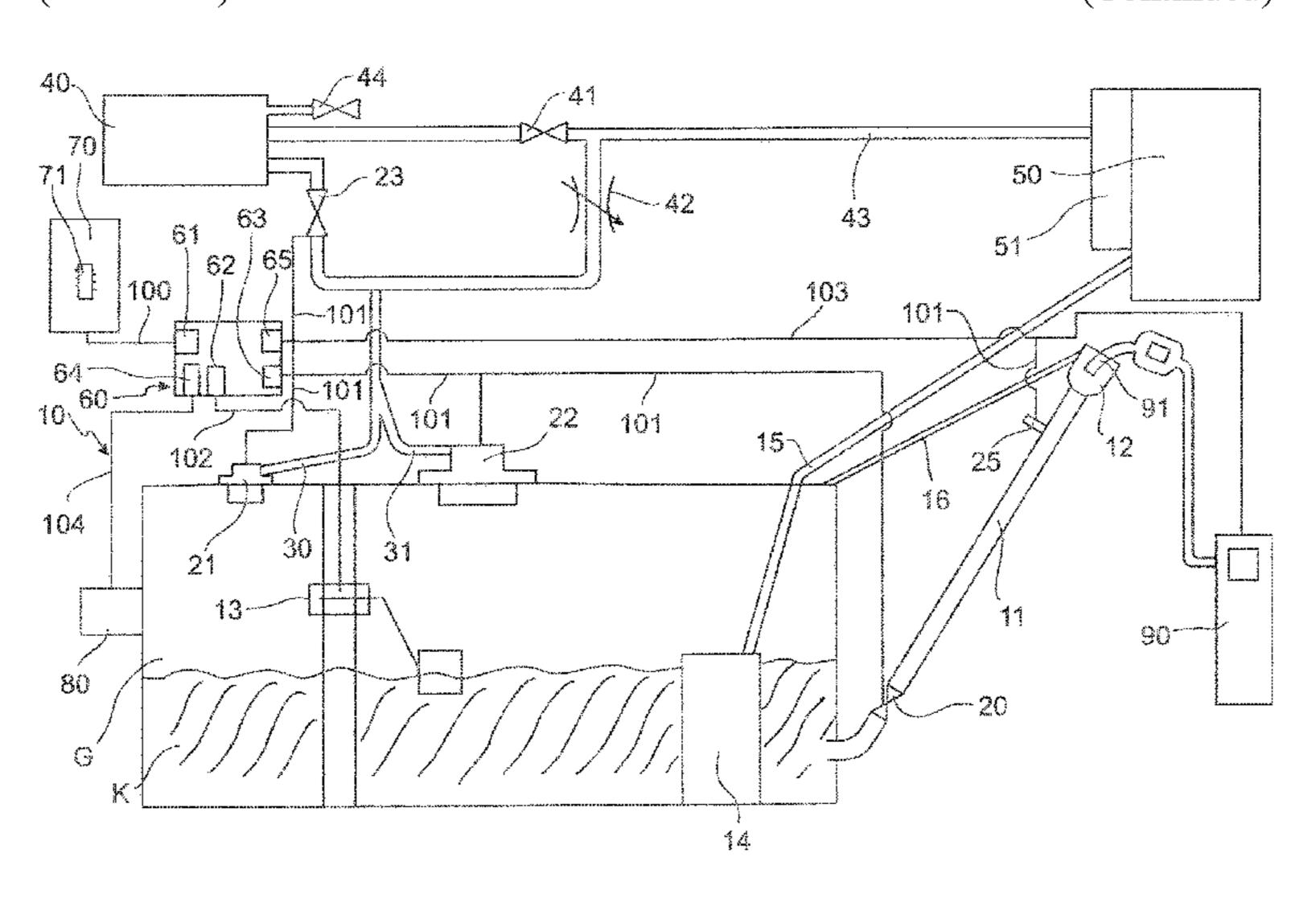
actuator via the first data exchange connection upon receiving data which represent a predetermined fill level of the operating fluid container; and the actuator initiates the termination of a filling procedure of the operating fluid container upon receiving the filling stop signal.
