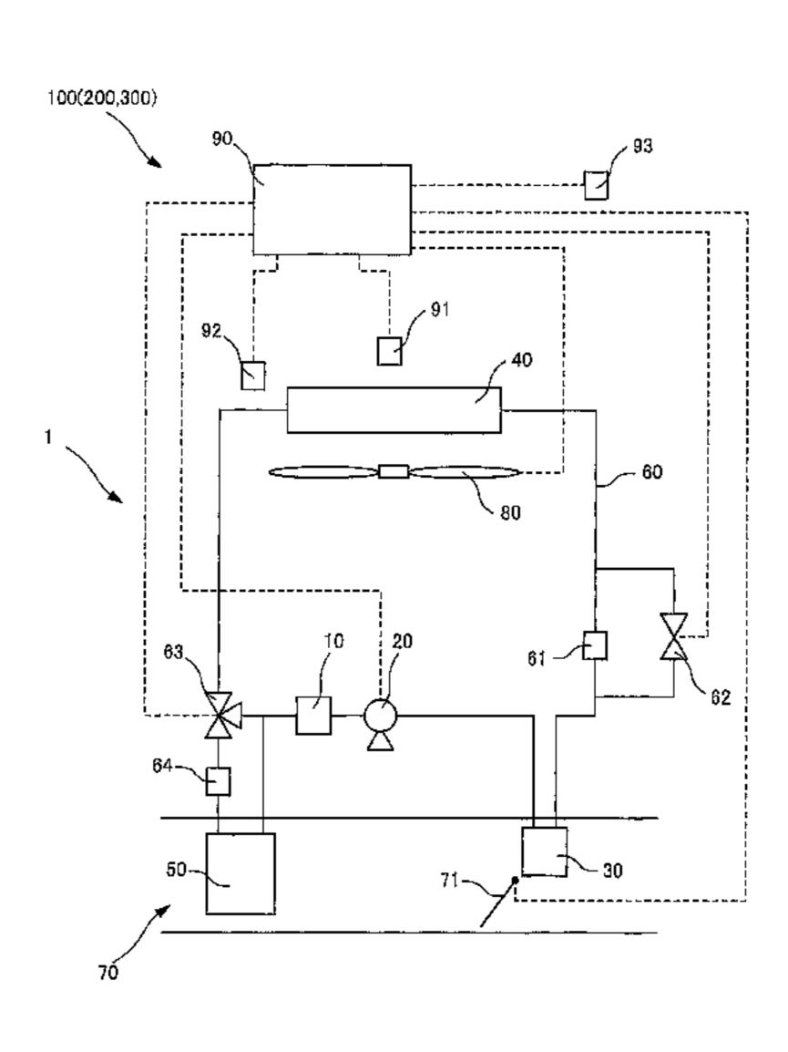
frost formation determination unit that determines that frost formation is caused on the external heat exchanger on the basis of the elapsed time to of a state in which the temperature difference  $\Delta T$  is equal to or larger than a frost-formation temperature difference at which the frost formation may be caused on the external heat exchanger.
