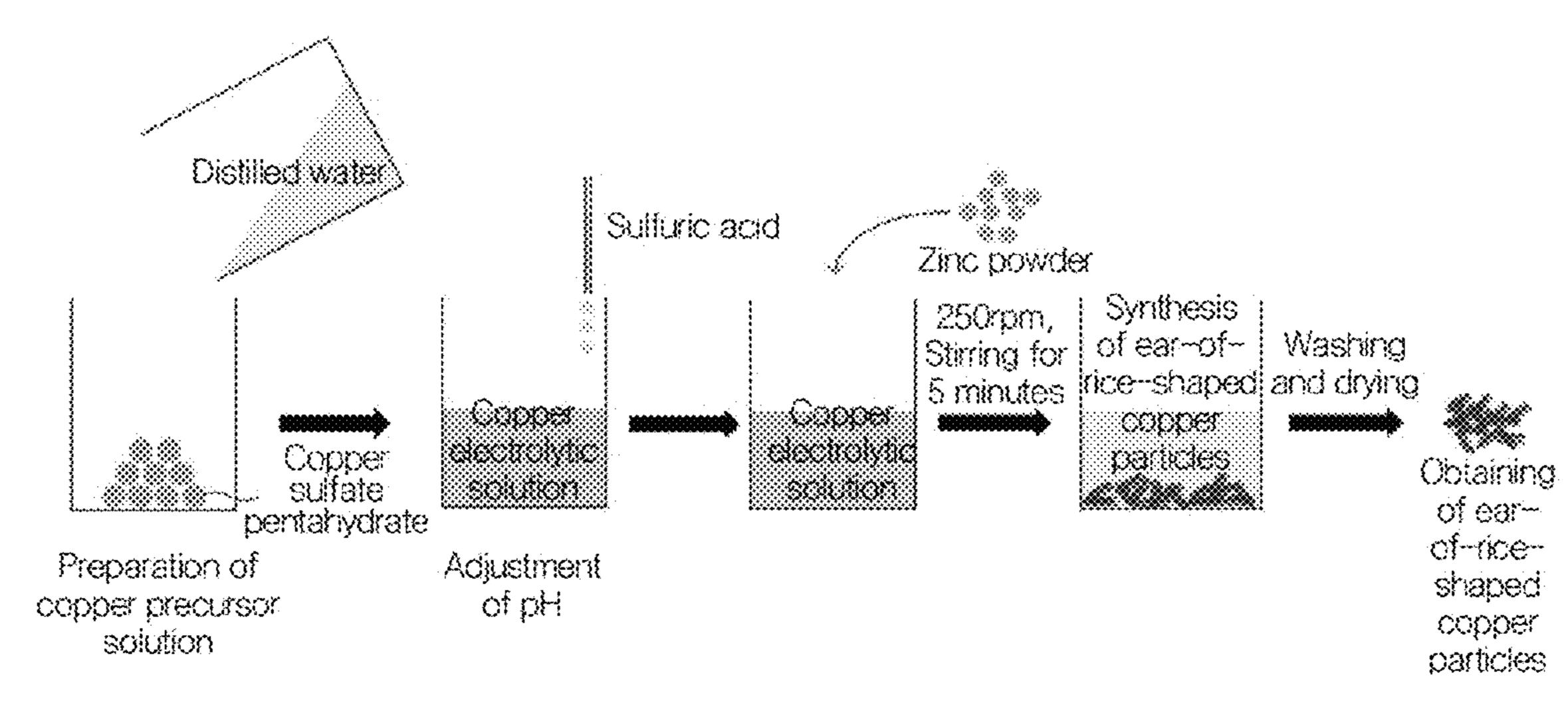
mined time, and a fifth step of separating, washing, and then drying the synthesized ear-of-rice-shaped copper particles.
