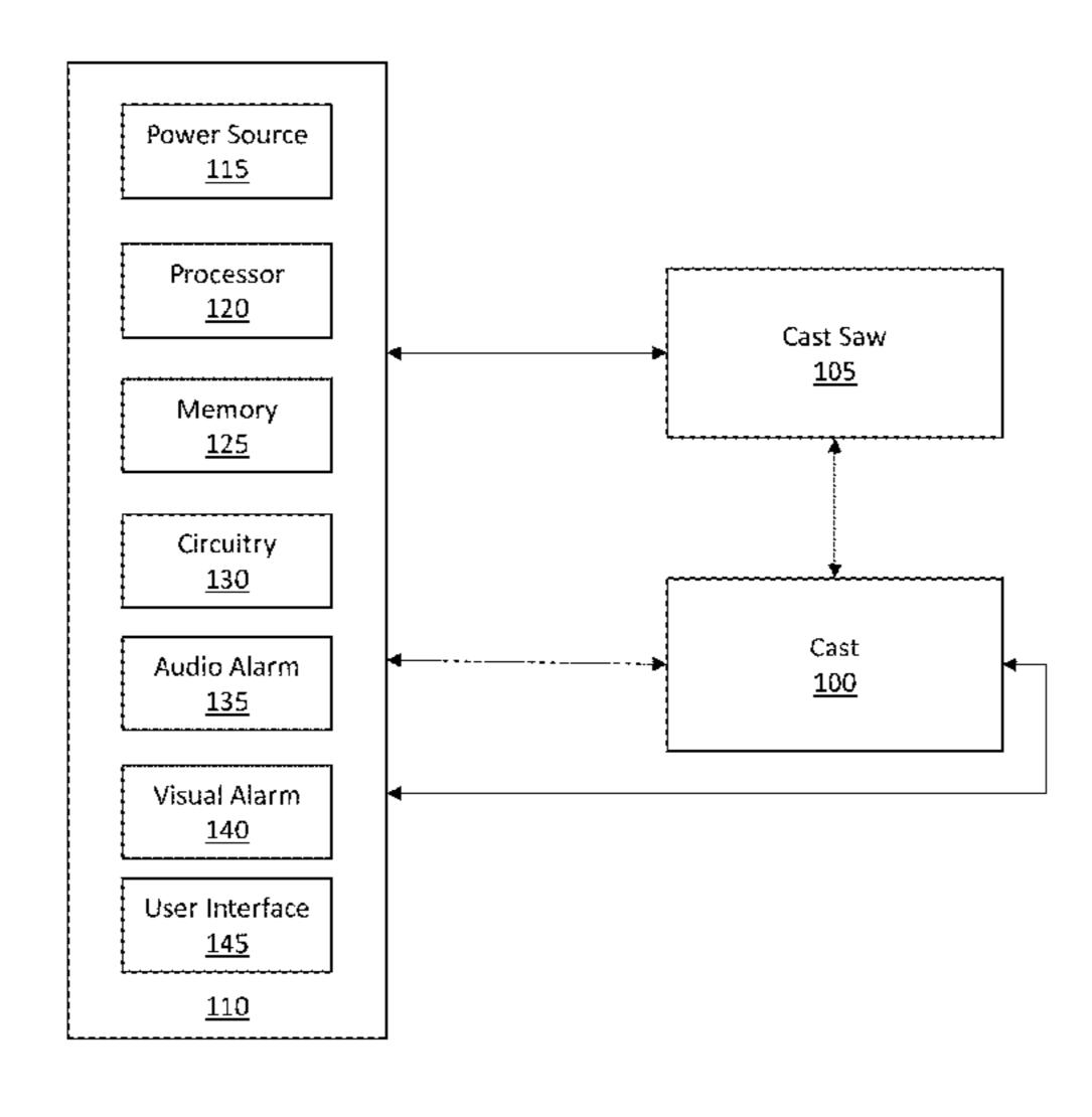
sor is further configured to activate an alarm to warn a user of the cast saw that the saw blade is in contact with the conductive layer.
