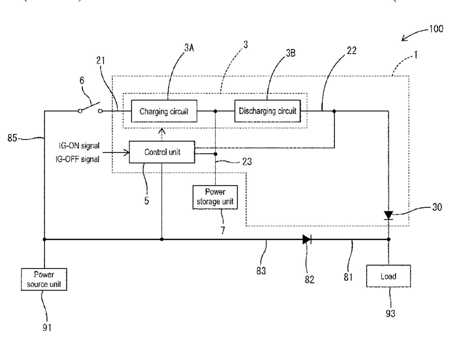
lower than a voltage that is applied to a power path in the case where a power source unit is fully charged, and a diode (element unit) that is provided between the power path and the output-side conduction path.
