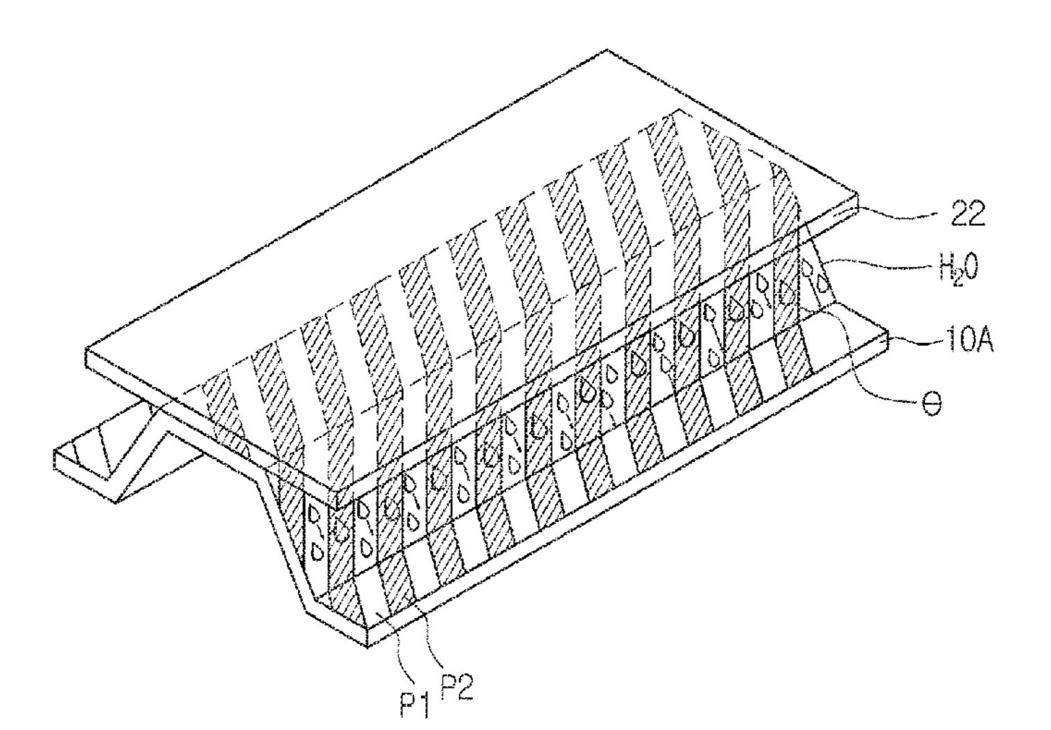
of Cr, 0 to 0.6% of V (excluding 0), 0 to 0.5% of Ti (excluding 0), 0 to 0.5% of Nb (excluding 0), and the remainder comprising iron (Fe) and other unavoidable impurities, wherein a plurality of patterns may be formed on a surface of the stainless steel in a direction that is inclined with respect to a rolling direction, and the plurality of patterns are arranged repeatedly in the rolling direction.
