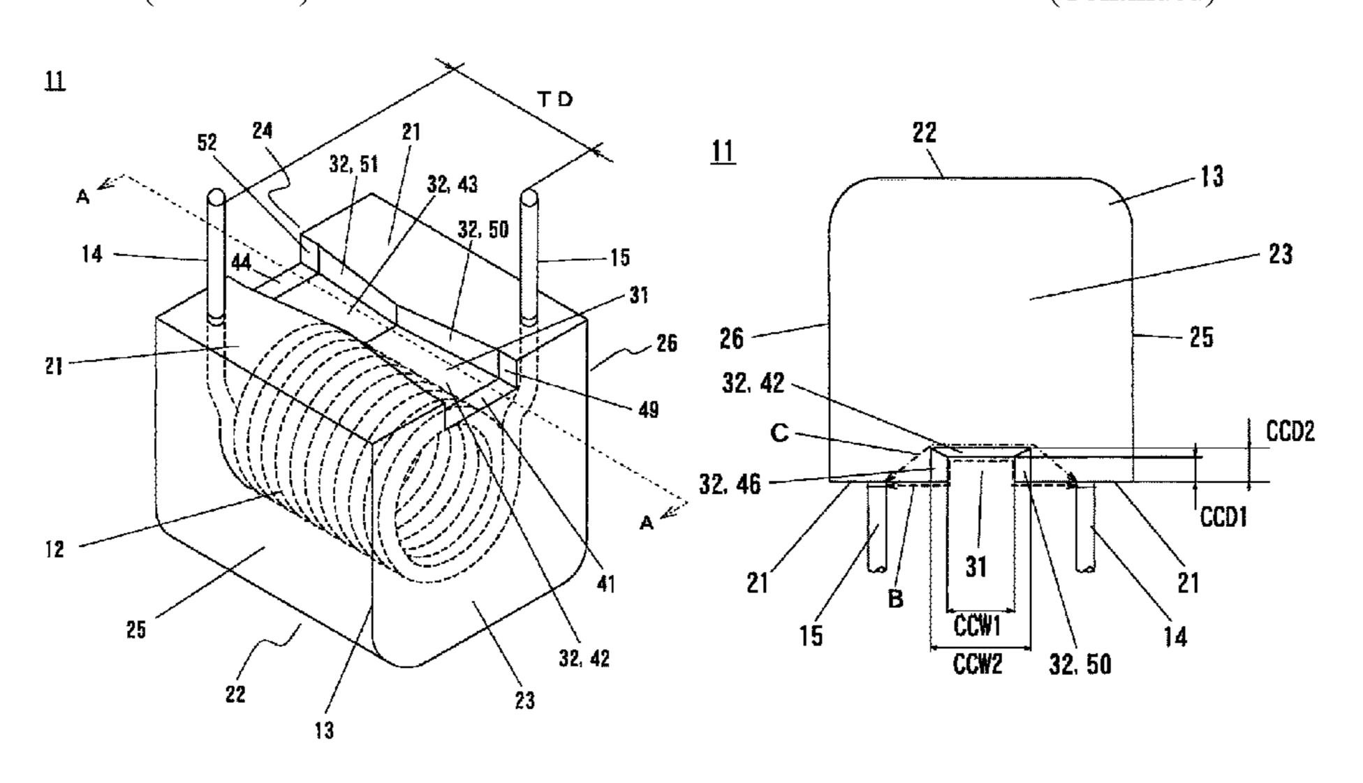
bottom surface. A line along the bottom surface extending from a position at which the first terminal protrudes to a position at which the second terminal protrudes is longer than a straight line extending from the position at which the first terminal protrudes to the position at which the second terminal protrudes.
