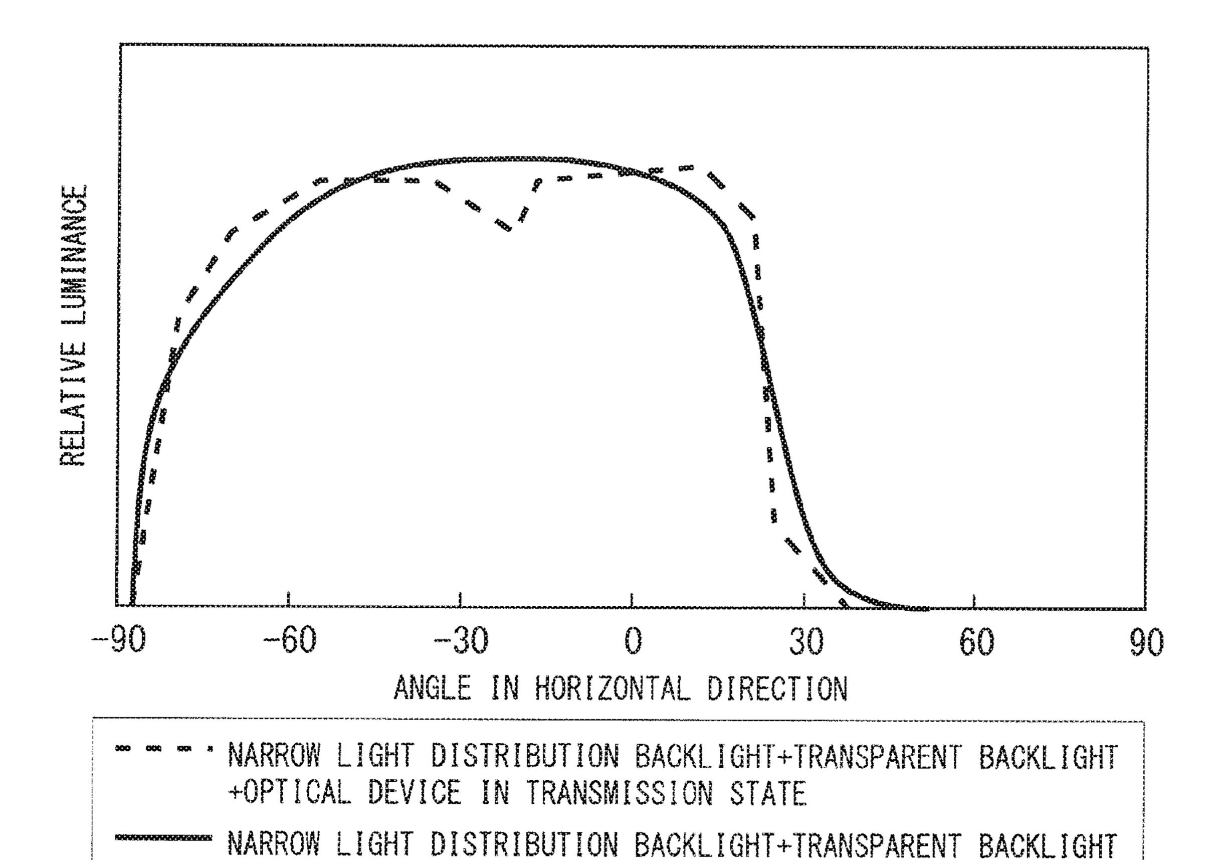
+OPTICAL DEVICE IN SCATTERING STATE
