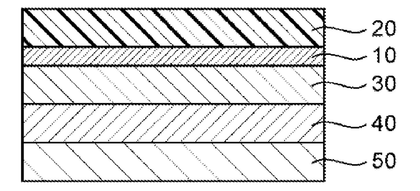
first optical compensation layer, the second optical compensation layer, and the third optical compensation layer shows a refractive index characteristic of nx>nz>ny.
