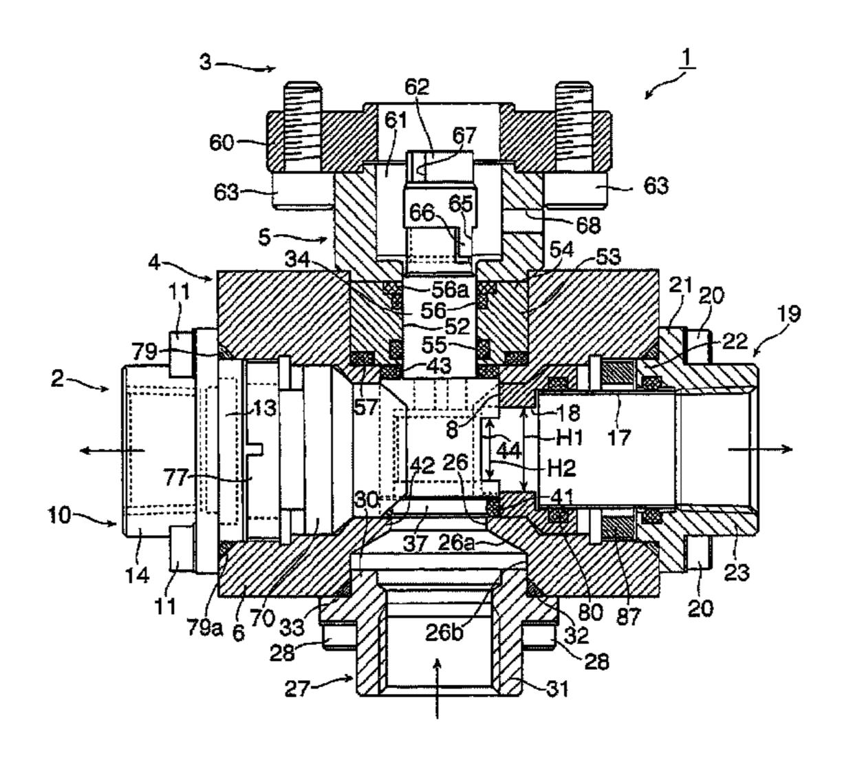
apply pressures of the fluid leaking through a gap between the valve body (34) and the valve seat (8) to the first and second valve port forming members (70) (80) so as to suppress shift of a position of the valve body (34) when the valve body (34) opens and closes the first valve port (9) and the second valve port (18); and drive means (3) for driving the valve body (34) to rotate.
