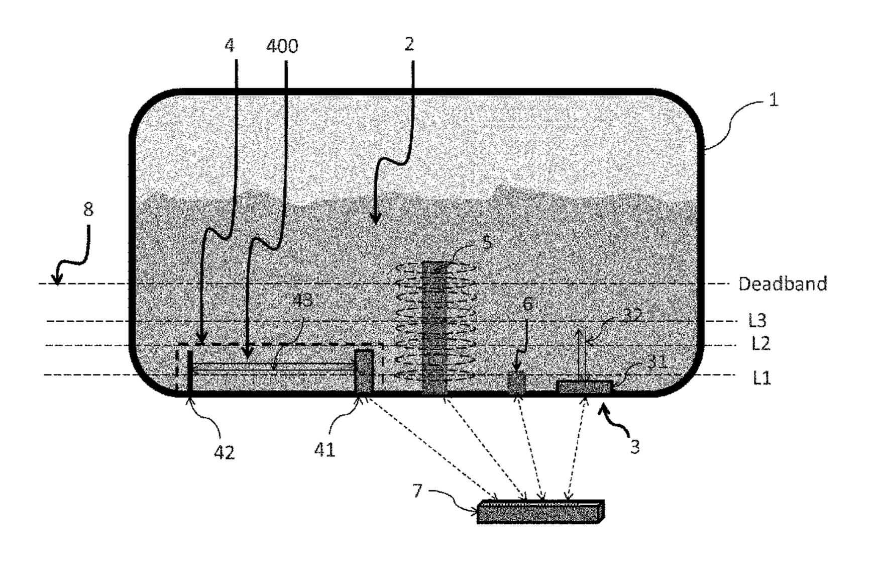
formed by said first ultrasound subsystem (S10); —when it is detected that the measurement of said first ultrasound system is not valid: (a) checking (S22) the validity of the measurement performed by said second ultrasound subsystem; (b) determining (S24, S25, S26) a quantity of liquid, which quantity being based on a result of the validity check at step (a).
