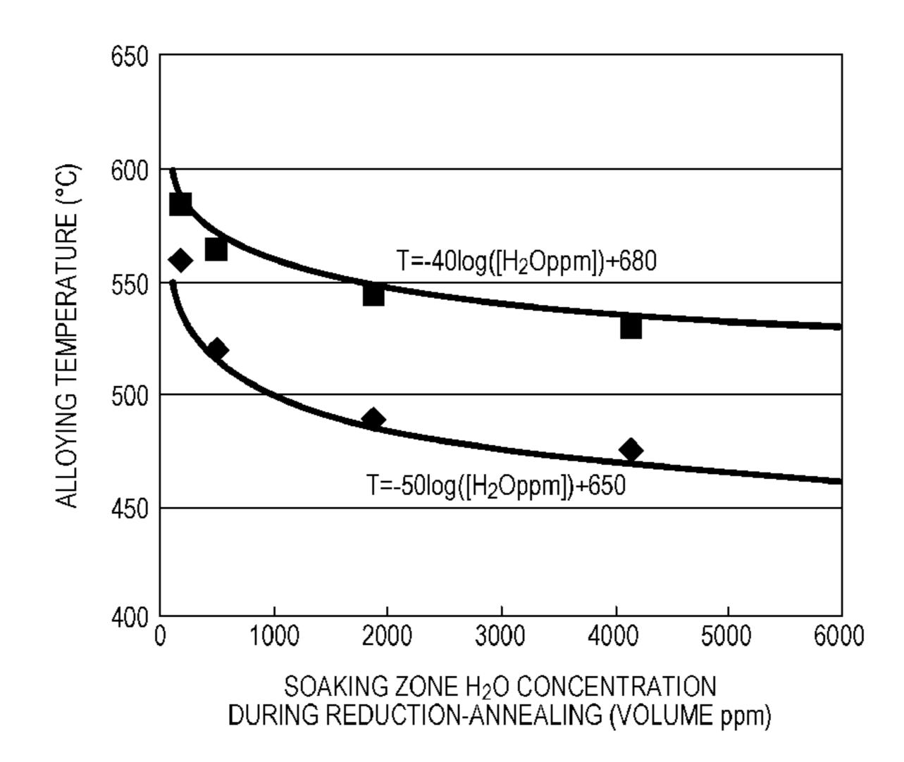
concentration of less than 1000 ppm by volume and a  $\rm H_2O$  concentration of 1000 ppm by volume or more. The method also includes reduction-annealing in which the steel sheet is heated at a heating rate of 0.1° C./sec or more to a temperature of 650 to 900° C. in an atmosphere having a  $\rm H_2$  concentration of 5 to 30 vol % and a  $\rm H_2O$  concentration of 10 to 1000 ppm by volume.
