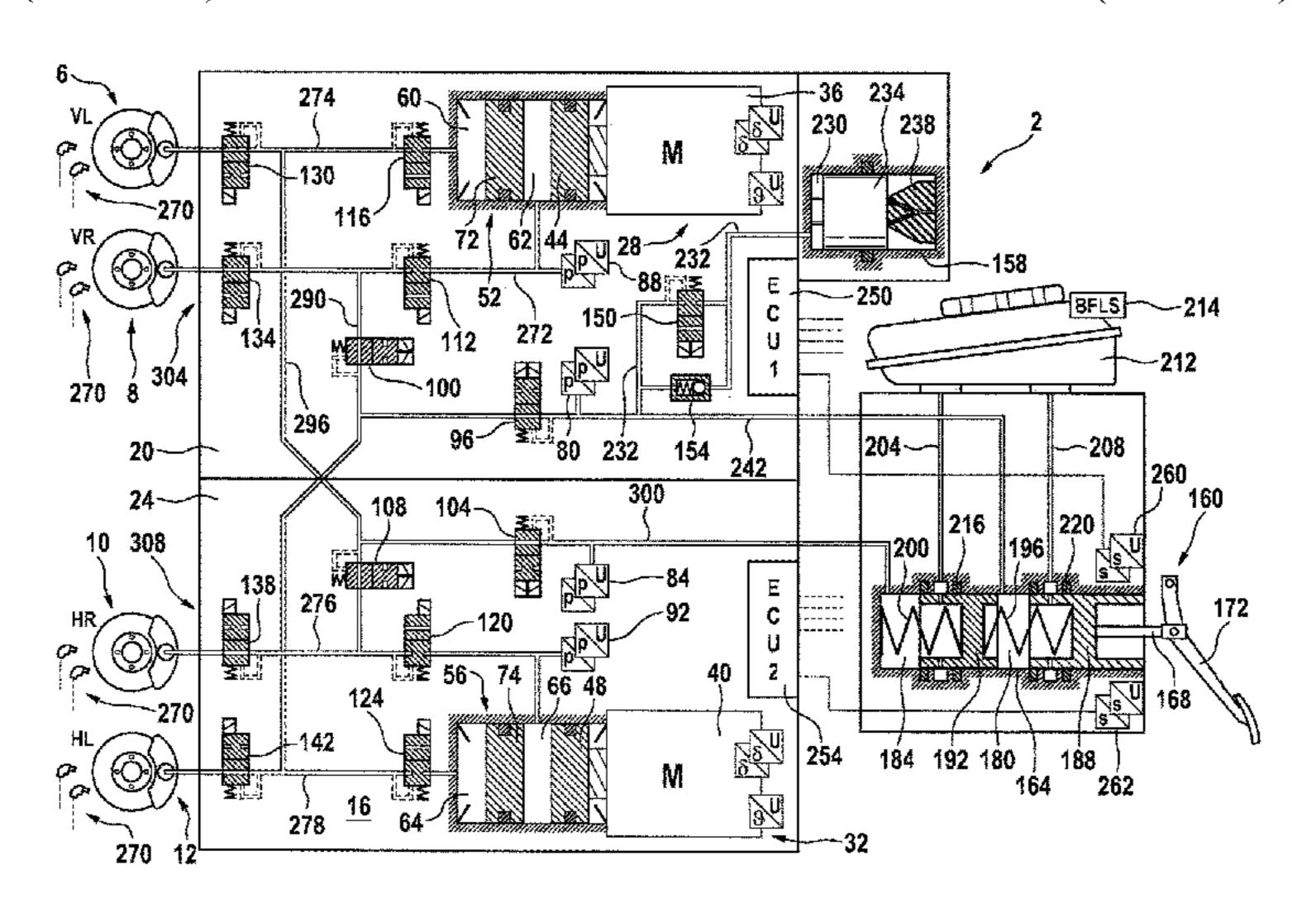
normally open isolating valve, connects the first wheel brake line of the first brake circuit to the first wheel brake line of the second brake circuit. A second hydraulic line, with a normally open isolating valve, connects the second wheel brake line of the first brake circuit to the second wheel brake line of the second brake circuit.
