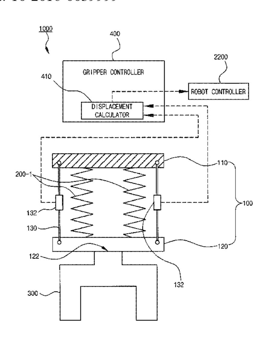
mount. A first end of the passive compliance part is fixed, and a second end of the passive compliance part is configured to be transformed. The displacement measuring element is equipped to the passive compliance part, and measures displacement due to transformation of the passive compliance part. The gripper mount is connected to the second end of the passive compliance part, and has a gripper part gripping a component.
